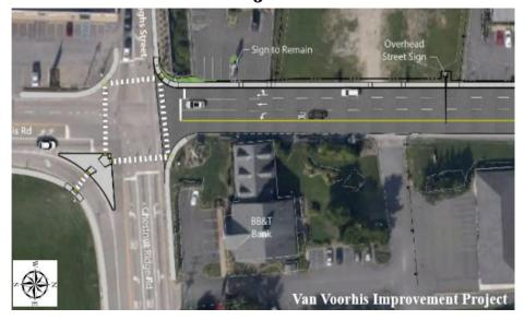
The Van Voorhis Improvement Project is expected to start construction soon; this project will improve traffic operation, roadway safety, roadway drainage, and walkability. Improvements include targeted widening for turn lanes, geometric curve improvement, wider lanes, sidewalk installation, paved shoulders, and bridge replacement.
